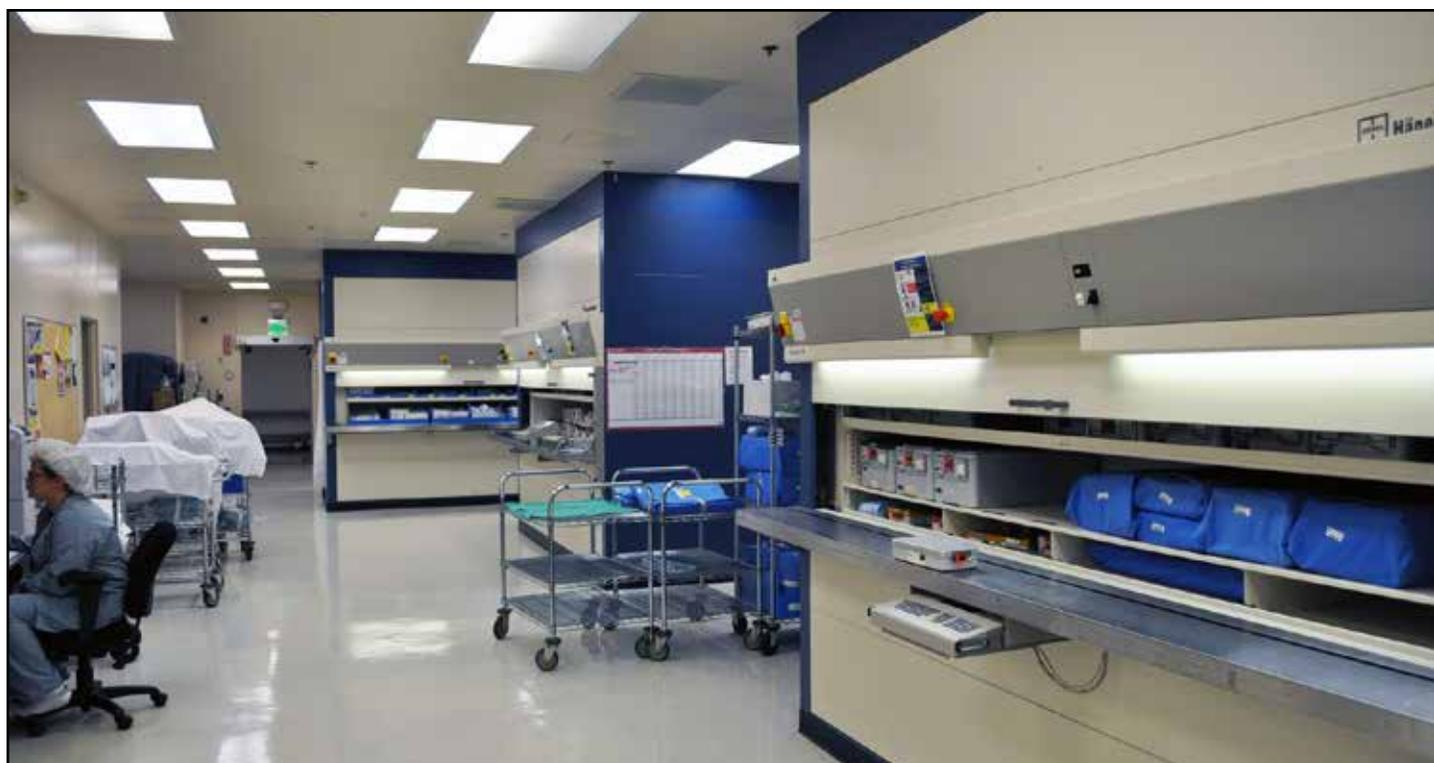
*AFTER: Rotomat® Storage Carousels are fully enclosed, allowing storage floor to ceiling that is secure and protected. Automation and inventory management ensure that proper inventory levels are maintained and that items do not expire. Carousel shelves are customized to suit individual needs, avoiding stacking and ensuring ideal storage conditions.*
